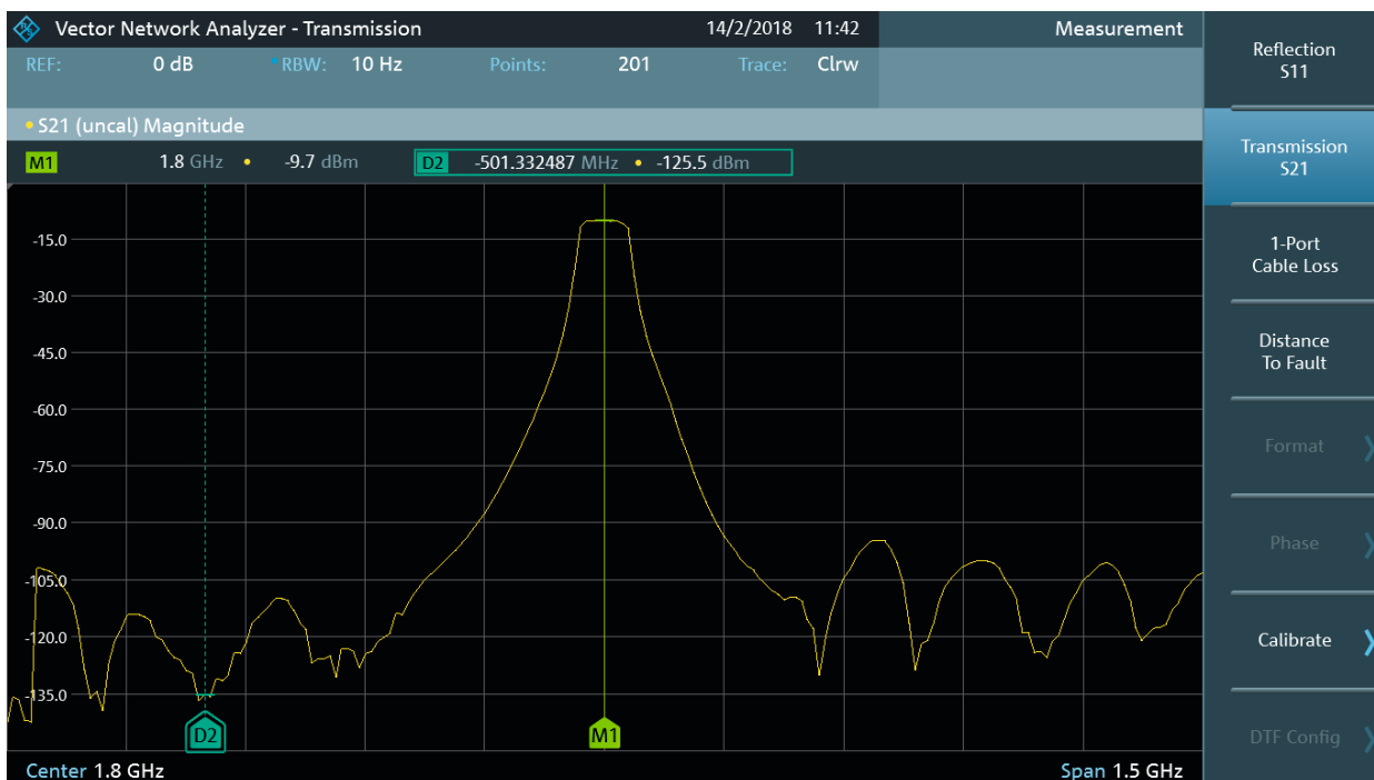
R&S®FPC1500 S_{21} scalar transmission measurement with the R&S®FPC-K42 option.
