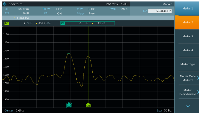
R&S®FPC-B22: high sensitivity with internal preamplifier.
