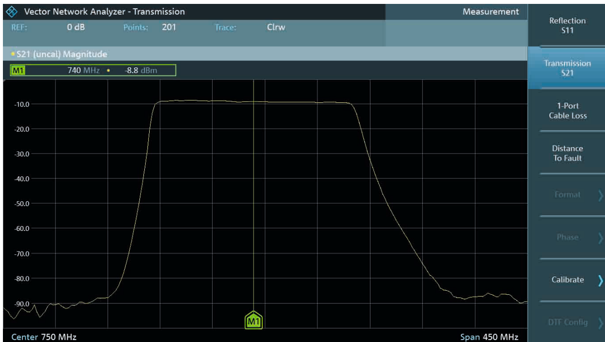
R&S®FPC1500: tracking generator measuring a filter.
